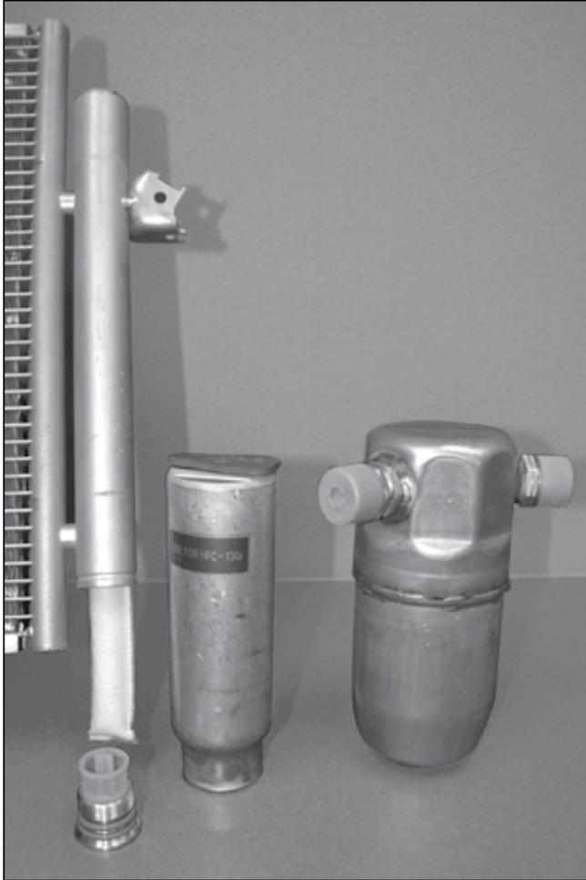
*The only way to remove significant moisture from a system is to replace the desiccant. Not only that, most compressor supplier's warranties require that the R/D, A/D, or desiccant be replaced when one of their compressors is being installed.*
