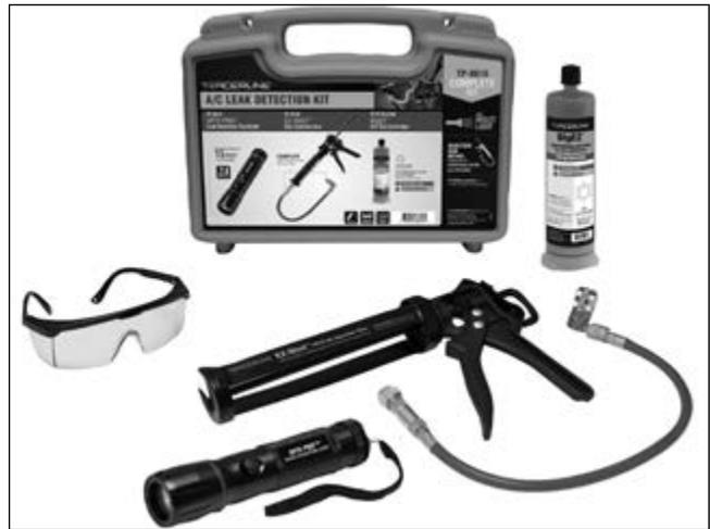
A typical UV dye leak detection kit contains dye, a dye injector (or some other type of tool to introduce dye to a system), a UV flashlight, and the correct goggles for the dye being used. Always wear the goggles to protect your eyes from the UV light. This kit also contains a special cleaner to remove traces of the dye after the leak is repaired.
