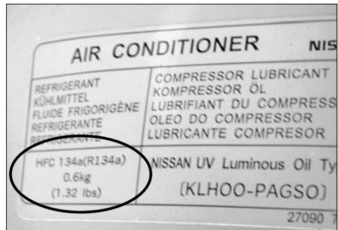
Infiniti (M45) label shows refrigerant capacity in pounds and kilograms, but with no tolerance listed.
