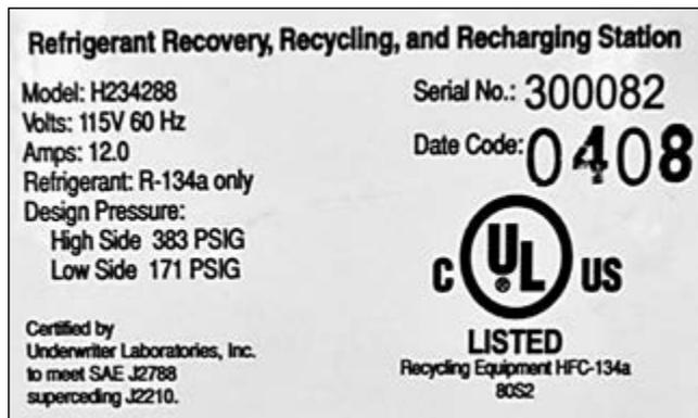
The refrigerant R/R/R machine label above states "certified . . . to meet SAE J2788 superseding J2210."
