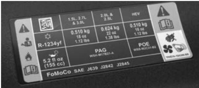
A vehicle's A/C system information label lists the type of lubricating oil that the system requires.
