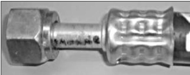
*Assembly crimped, rotated and re-crimped.*
