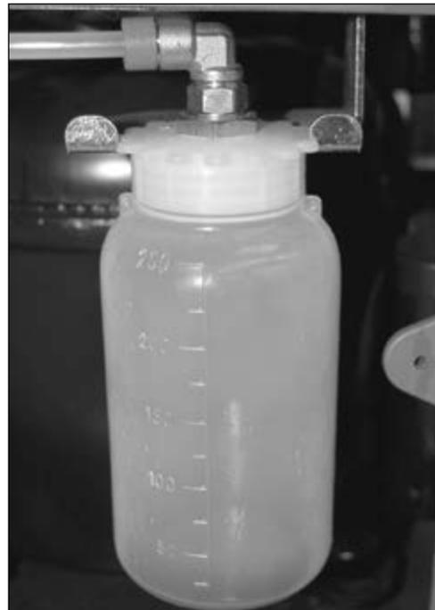
Here is a typical recovery machine's oil recovery reservoir. It should be emptied before each recovery operation, then checked when recovery is completed to see how much (if any) oil was removed from the system during recovery. If oil was removed, that same quantity of fresh new oil of the type the system requires must be reinstalled in the system before it is put back into operation.
